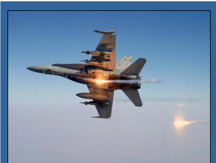
F/A-18 firing countermeasure flares during a system test (DoD public domain photo by Lt. Peter Scheu, USN)
