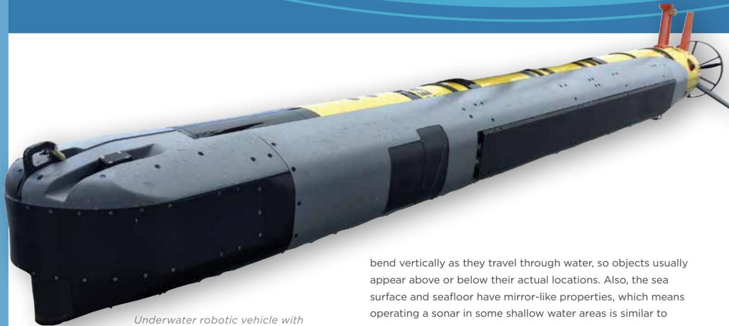
*Underwater robotic vehicle with forward and side looking sonars.*
