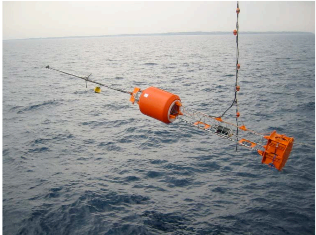
Recording electronics in tower section. 802.11g antenna on top of mast.
